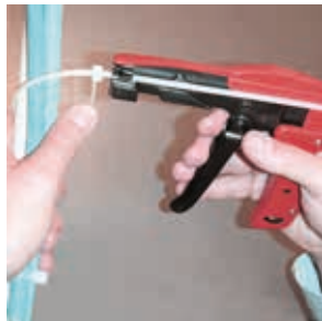
Grip the cable tie with the tool.
