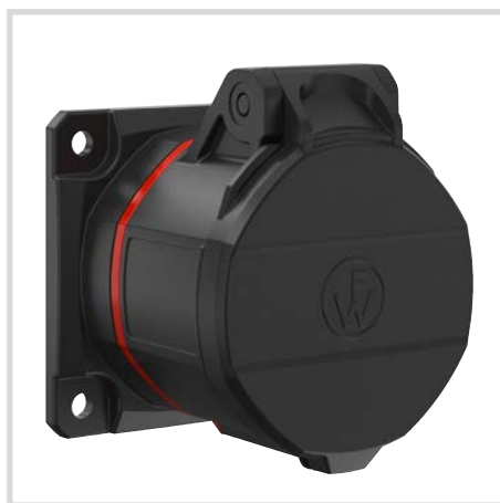
CEE NEO panel socket, straight 5 x 16 A | 6 h | IP54 screw terminal or cage clamp connection
