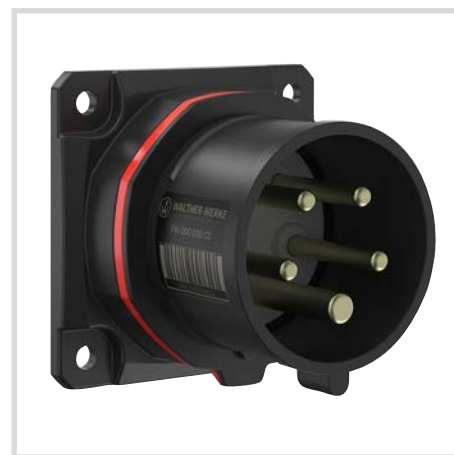
CEE NEO panel mount appliance inlet, straight, 5 x 16 A | 6 h | IP54 screw terminal or cage clamp connection
