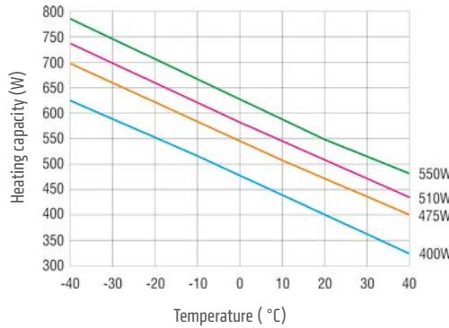
Heating capacity / Ambient temperature diagram
